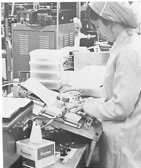
Kris Peterson operates a folding machine which forms the protective and reusable envelopes in which the Markette I is contained.
