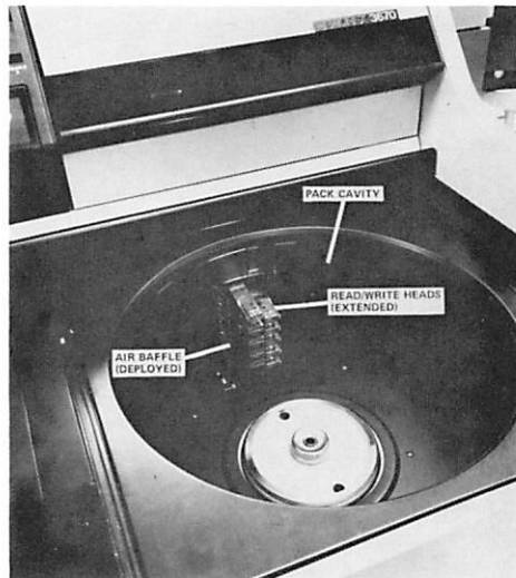
The self-actuating air baffle, the comb-like device shown extended in the photo at left, allows utilization of the spinning disc pack to pump filtered air throughout the drive, eliminating the need for additional fans or
