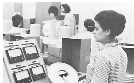
After assembly, plastic computer reels are inspected and tested before final packaging by Elena Heinzman, assembler.
