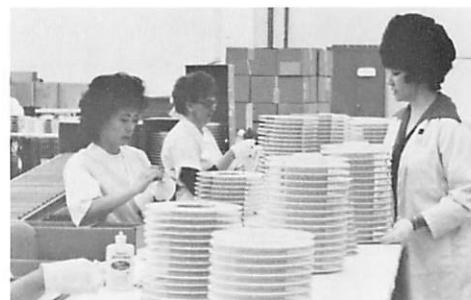
Visual inspection and cleaning is performed on the computer reels by (l to r) Susie Enyeart, Esperanza Ferra and Mandy Eldred, assemblers.
