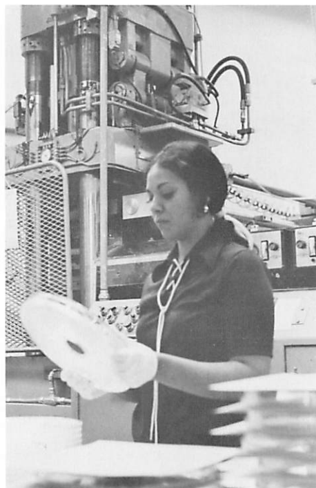
The tape canister is inspected as it comes from the vertical molding machine by Jane Aguinaga, molding machine operator.
