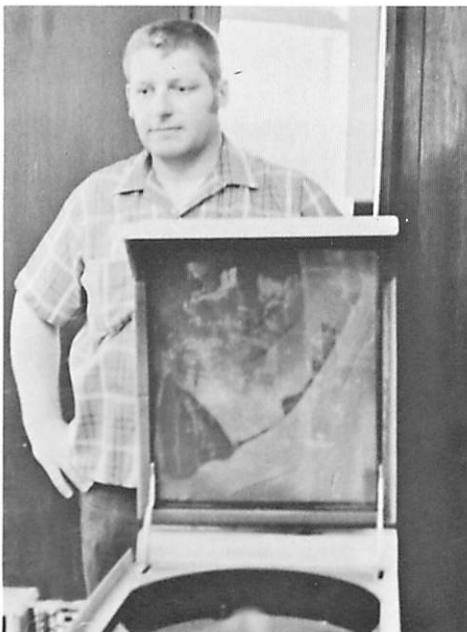
Surveying damage to Memorex equipment following tropical storm Agnes is Jim Silver, senior Memorex field support rep, Syracuse, N. Y. Note normally clear 630 drive cover is opaqued by silt after the flood.
