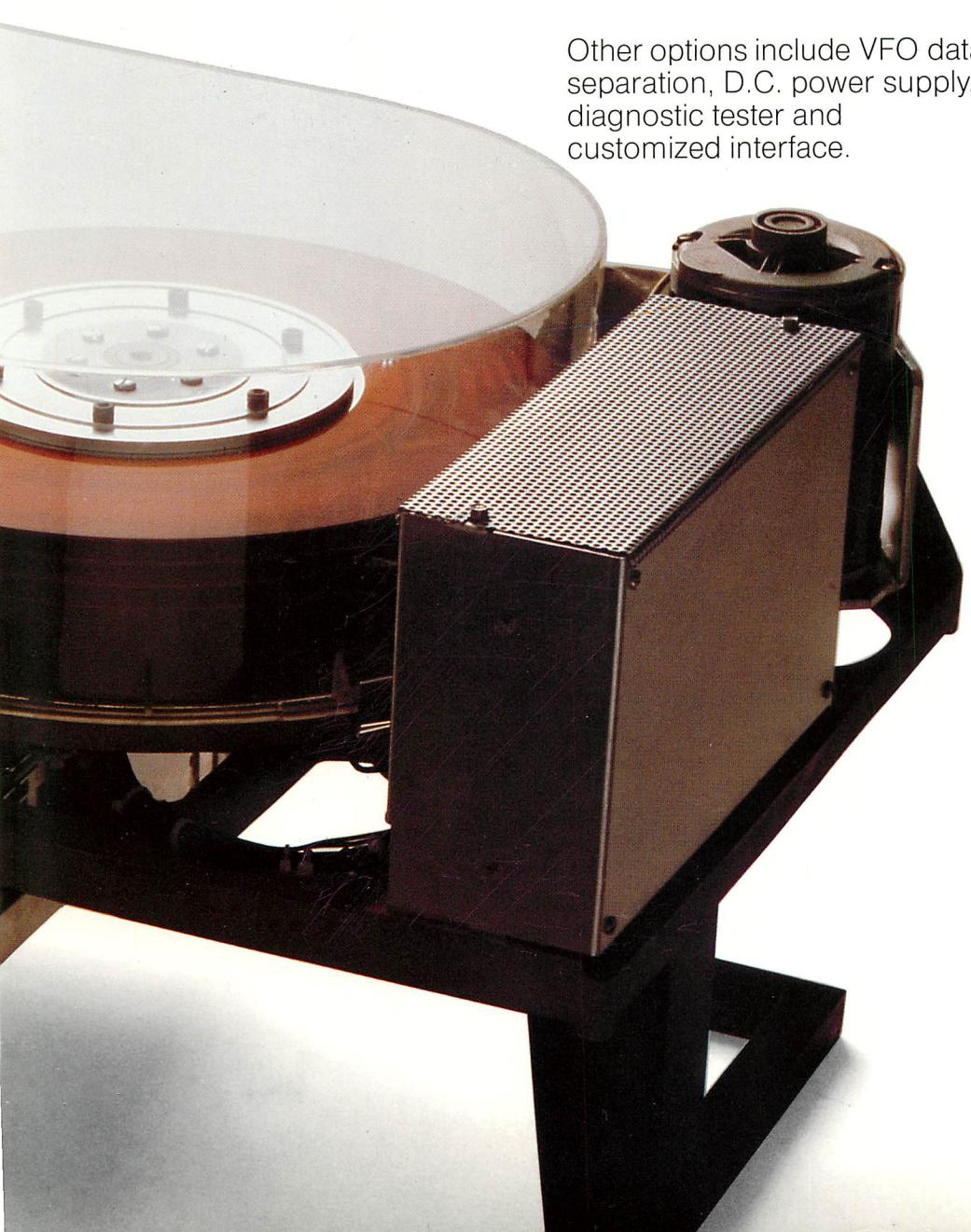
Access speed. Twin heads for each data surface provide the same fast access throughout the capacity range. Access time is as short as 7ms, averages 32ms, and is never longer than 75ms. Average access for a typical removable disc is 53ms; a flexible disc requires 300ms or more.
