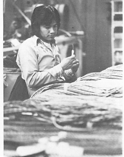
Mem-Mex employees put together dozens of types of wires to form the cables and harnesses that power Memorex disc drives.
