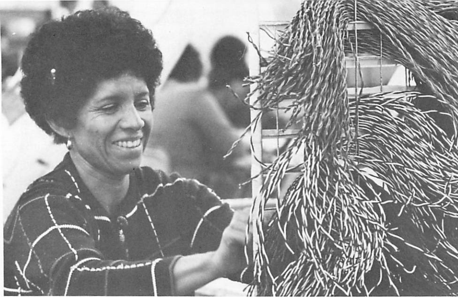
Mem-Mex employees put together dozens of types of wires to form the cables and harnesses that power Memorex disc drives.
