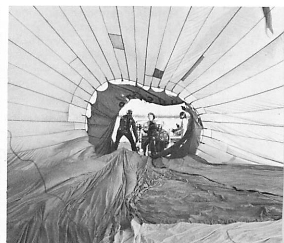
Farnham, center, inspects inside of rip-stop nylon balloon. Right, he heats air with propane burners to right balloon and prepare it for liftoff.
