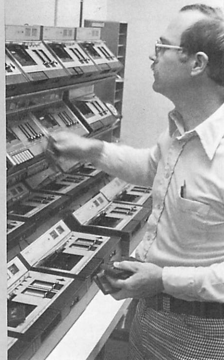
Senior Engineering Technician Dave Conway puts finished cassette tapes through series of tests on recorders in division's Quality Control Lab.
