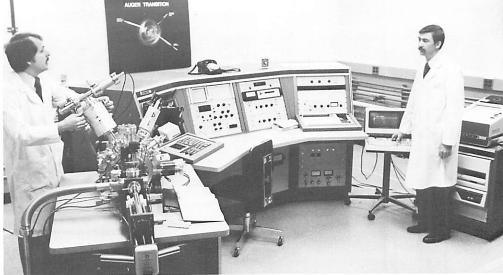
In SAM laboratory, Boynton, left, adjusts vacuum chamber, while Dodson uses visual display terminal. System also includes microprocessor, center, and small computer, far right.
