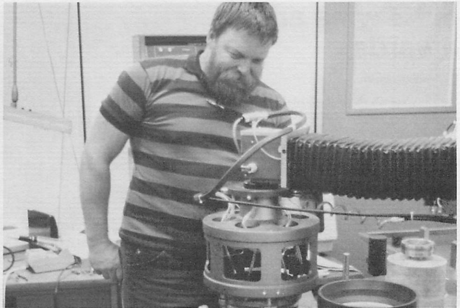
Robotics technician Rick Smith trains or programs Fared , one of Memorex's new disk stacking and assembly robots, to load disks into the head disk assembly hub with precise movements. The automated machines are about two months away from operating in a clean room environment.
