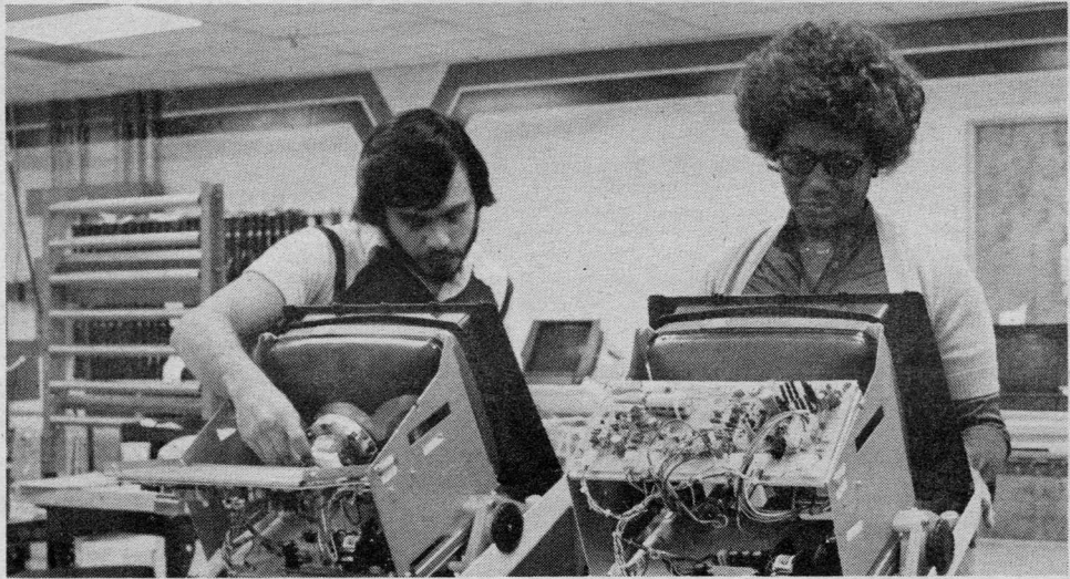
G. Rodriguez adjusts a terminal while L. Johnson performs a quality inspection.
