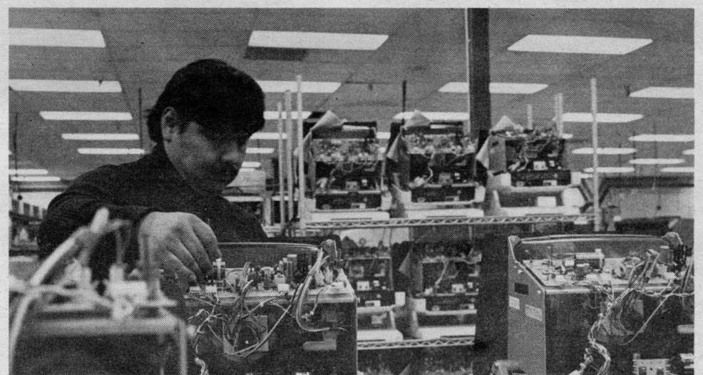
J. Donate uses a light meter to align a terminal.
