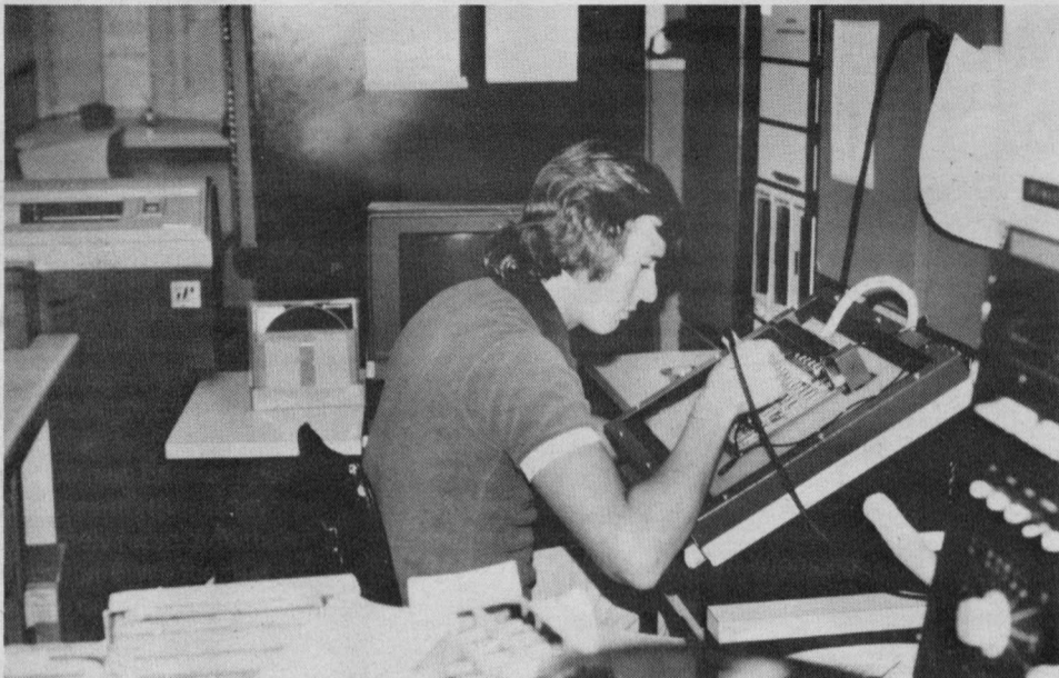
David Borowiec, Winnipeg industrial engineering technician, is shown using a logic probe to verify the logic integrity of integrated circuits.
