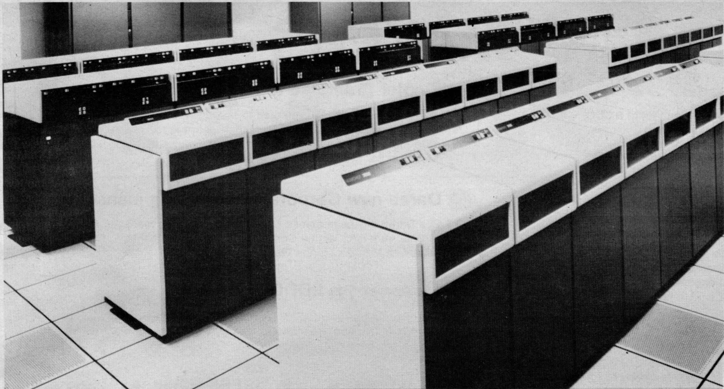
These random-access Memorex disc drive systems enable lawyers, executives and journalists to obtain information on any subject they choose without leaving their offices. Searching for specific words or phrases, the magnetic heads quickly locate material for display and printout on custom-designed timesharing terminals.
