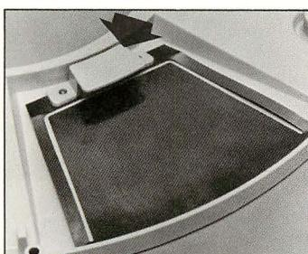
The air inlet port is stopped against a thick polycarbonate "brake" to minimize potential pollution.
