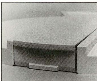
The "lap-butt" latch fits snugly against the latch frame and lower cartridge housing for greater sealing reliability. Instead of heat staking, shafts that go into sockets are used to create spring-tension hinges for more positive sealing. Guide ribs with sloping faces help assure positive closure.
