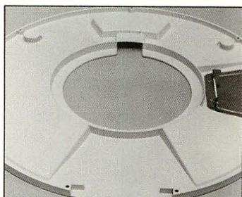
The cartridge has no bosses to keep the disc from sliding or floating during transport or when roughly handled.
