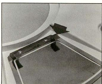
The air inlet port and stop are metal against metal and thus, debris prone.
