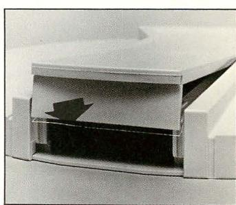
The thin plastic membrane can break or deform after usage. It is affixed to the latch by heat stake rivets which produce flashings that can flake off and become debris.
