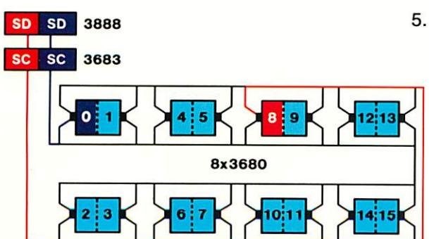
MAPS insures that all 15 actuators in a string are available for a second Input/Output operation. This compares to the IBM dynamic pathing selection (DPS) system which only allows the second Input/Output operation to go to 12 of the remaining 15 actuators.
