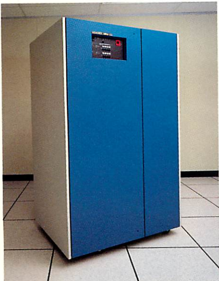
The Memorex 3888-23 Disk Cache Controller increases the performance of the 3682 Subsystem by providing cache storage of up to 64 megabytes in eight megabyte increments.
