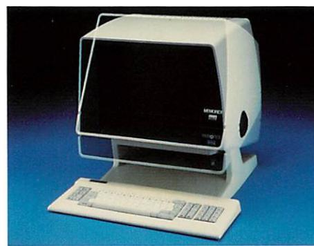
The 2078's monitor tilts and swivels to your most comfortable viewing position, and it can be easily removed from its stand to save space.
