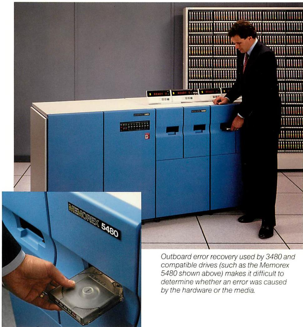
*Outboard error recovery used by 3480 and compatible drives (such as the Memorex 5480 shown above) makes it difficult to determine whether an error was caused by the hardware or the media.*
