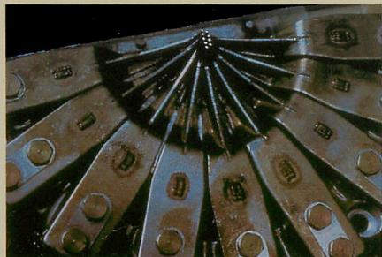
many printers won't. It operates quietly with a patented, long-life (over 500 million characters), stored-force flexhammer printhead that actually runs cooler at high speed. Features include:
