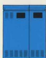
The 3698 contains the alternate controller functions and one disc drive. This provides access to the string as an alternative to the 3697.
