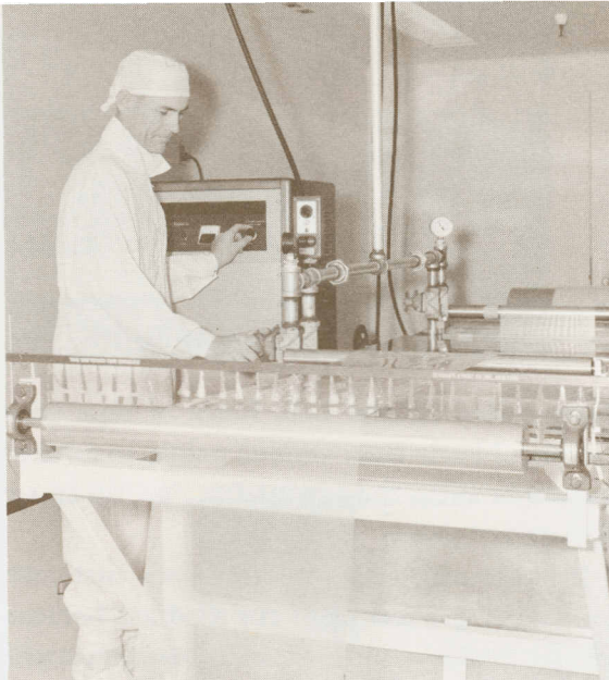
Ultrasonic cleaning system, designed by Memorex engineers, removes foreign matter from film base material before coating.
