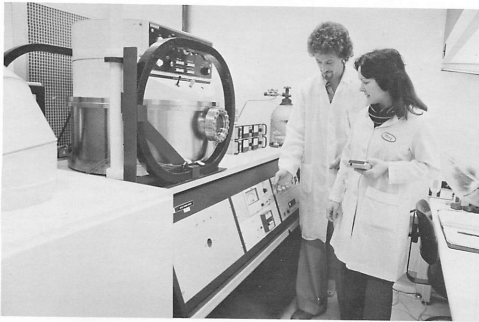
Two technicians work with the sputtering unit in the thin film lab. The sputtering unit is used for depositing thin film materials onto a substrate. The process allows 2,500 thin film heads to be made at a single deposition. This is substantially faster than making heads for the 3650, which are done one at a time.
