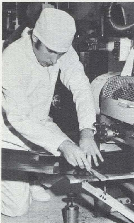
BOB WALZBERG marks the tape as he puts it on his slitter so he can tell its overall length within inches.
